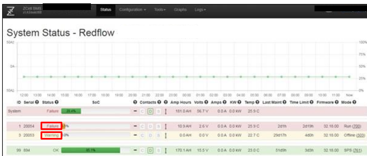
Figure 24: BMS interface showing warning and failure alarms on the Status page
