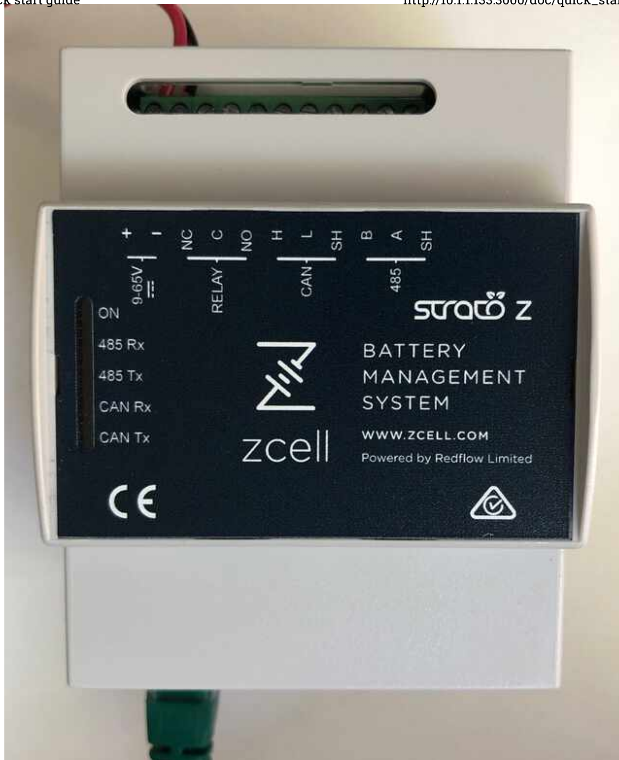
Figure 1: BMS terminal connections They are also labelled on the top panel.
